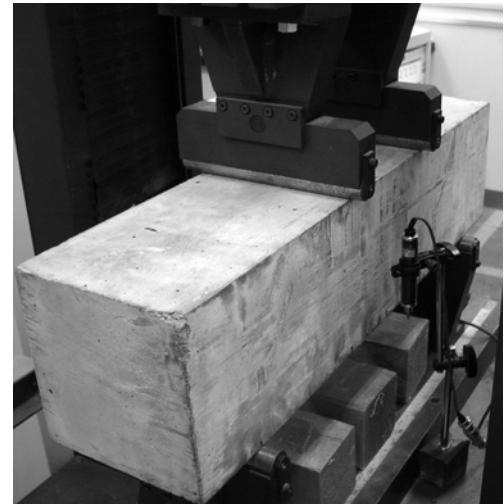
Figure 3. Four-point bending test
