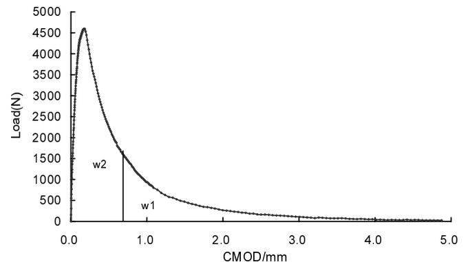
Figure 4. P-CMOD curve by wedge-splitting test.
