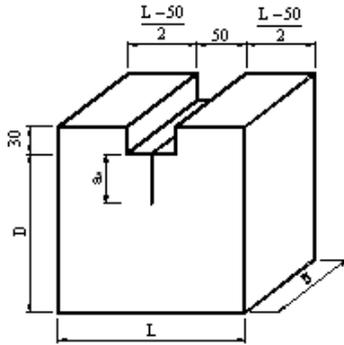
Figure 1. Geometry of wedge-splitting specimen (unit:mm).
