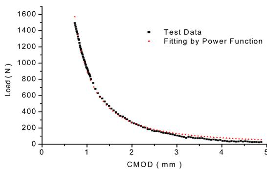
Figure 3. Comparison between the fitting tail section curve by exponential function and the corresponding tested curve.
