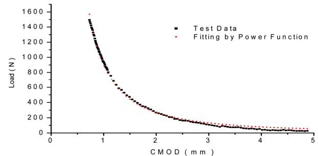
(c) Comparison between the fitting curve and the tested curve
