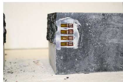
Figure 1. Experimental setup and a half-specimen with bonded strain gauges after testing (units in mm).
