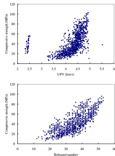
Figure 1. Variation of compressive strength with UPV and rebound number.
