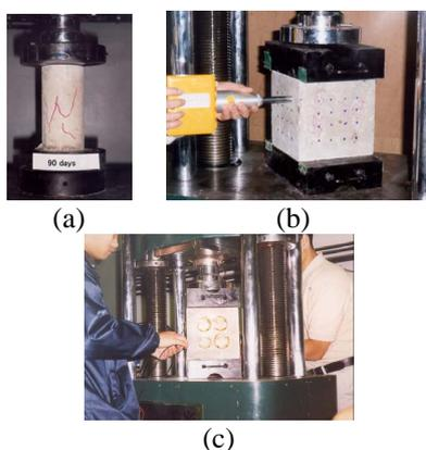
Figure 2. Experimental study (a) compressive test, (b) rebound hammer test, (c) UPV test.
