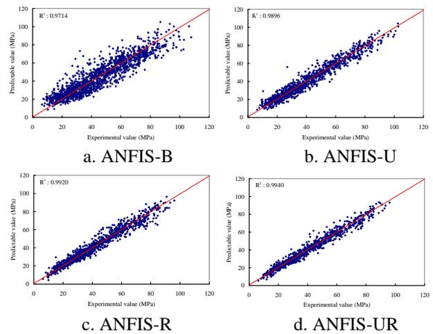
Figure 4. Comparison of experimental strengths with predicted results.
