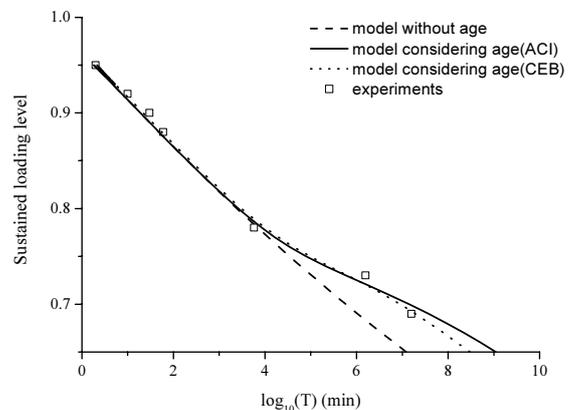
Figure 4. The relationship between loading level and failure time.
