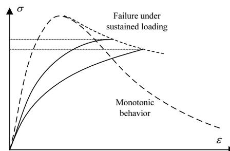
Figure 1. Sustained-loaded envelope for concrete in uniaxial compression (Rüsch, H. 1960).
