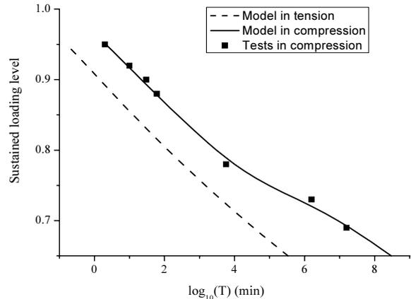
Figure 6. The relationship between tensile and compressive loading stress level and failure time.
