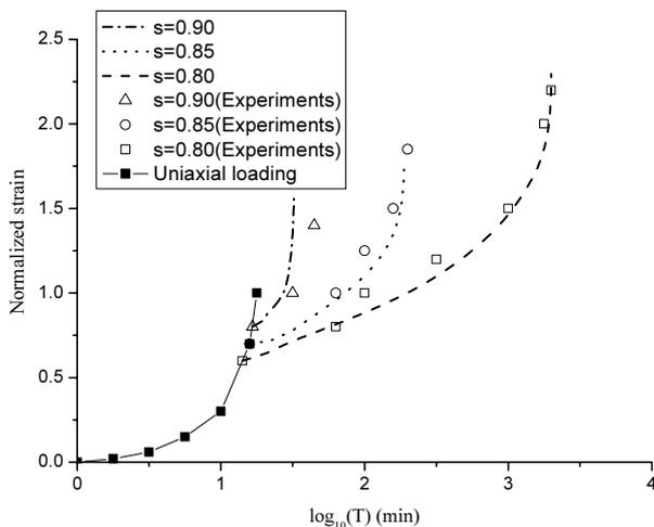
Figure 5. Strain variation with sustained loading time.
