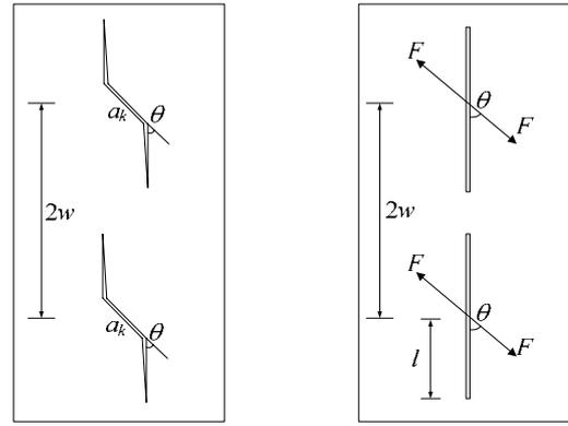
Figure 3. Periodical crack model of concrete.
