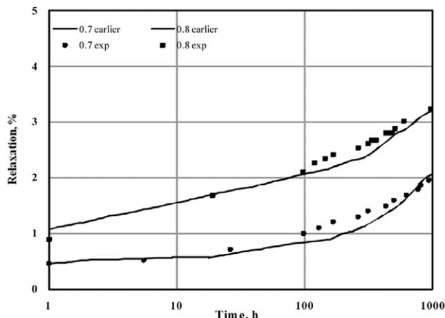
Figure 5. Comparison of experimental results with Erdelyi (1989) research.
