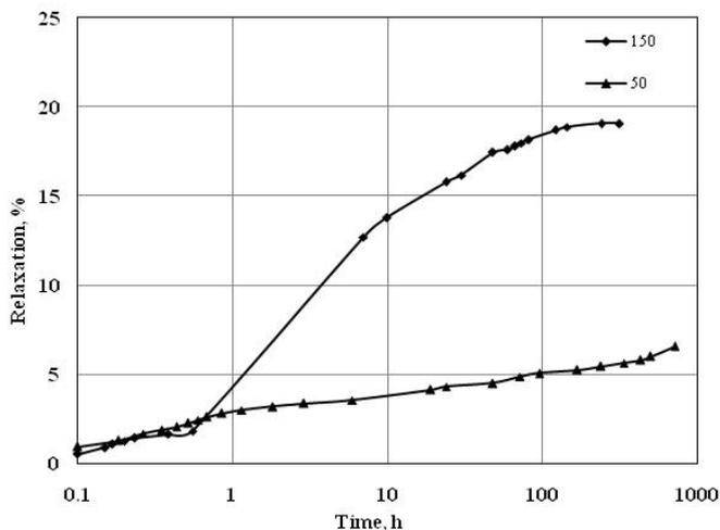
Figure 4. Relaxation loss at 50°C & 150°C at 0.7 initial prestress.
