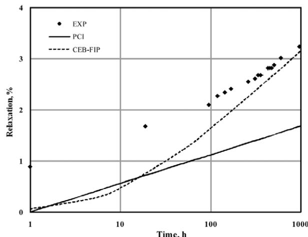
Figure 7. Comparison of experimental with PCI and CEB-FIP at 0.8.
