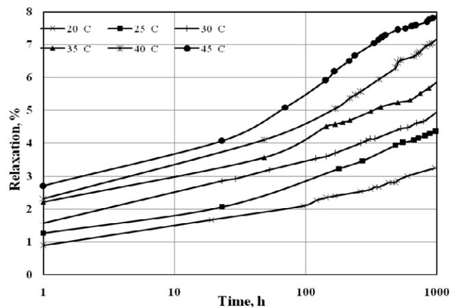
Figure 2. Relaxation vs. time at an initial prestress of 0.8.
