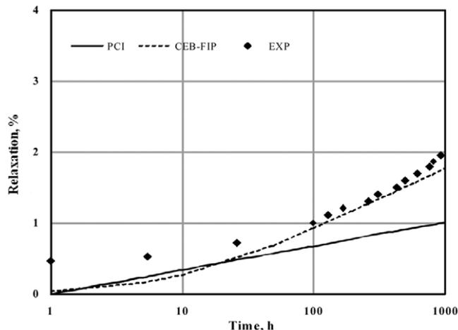
Figure 6. Comparison of observation with PCI and CEB-FIP at 0.7.
