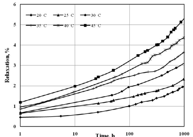
Figure 3. Relaxation vs. time at an initial prestress of 0.7.
