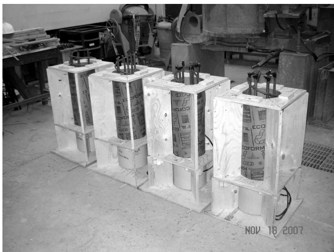
Figure 3. Formwork used in the production of the columns.
