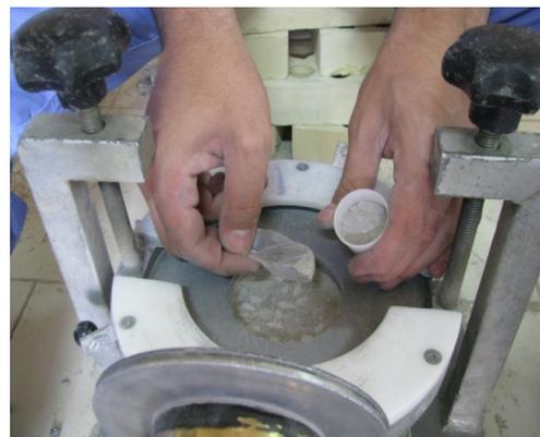
Figure 3. Sampling of concrete specimens using the Profile Grinder in exposure site.
