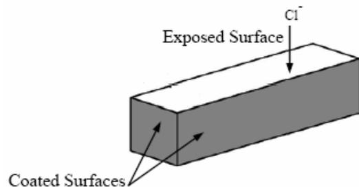
Figure 2. Typical concrete prism specimen and preparing the slice for powder sample.
