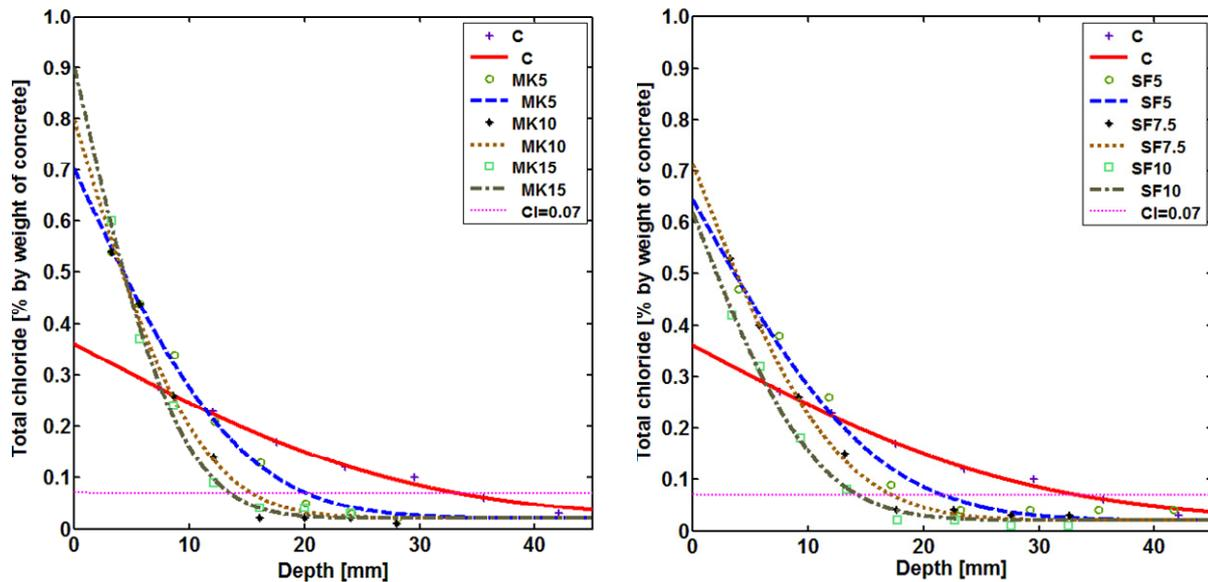
Figure 5. Chloride concentration profiles in tidal zone.
