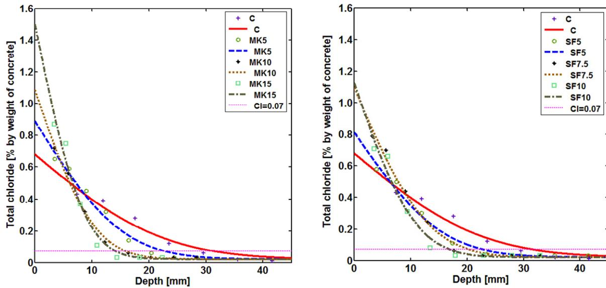
Figure 4. Chloride concentration profiles in splash zone.
