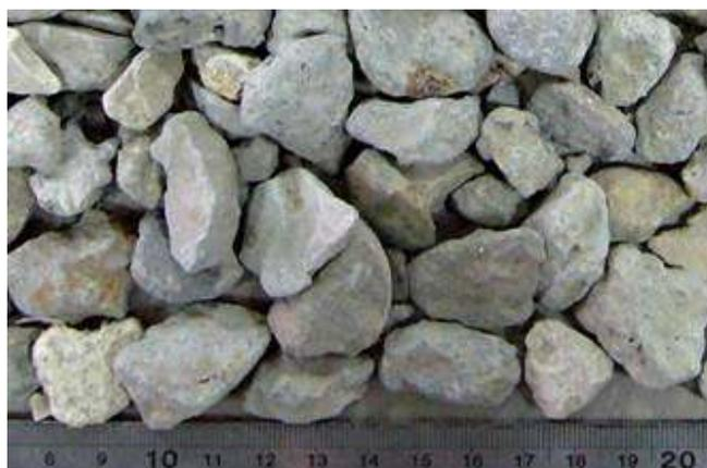
Figure 3 Recycled hardened mortar aggregate
