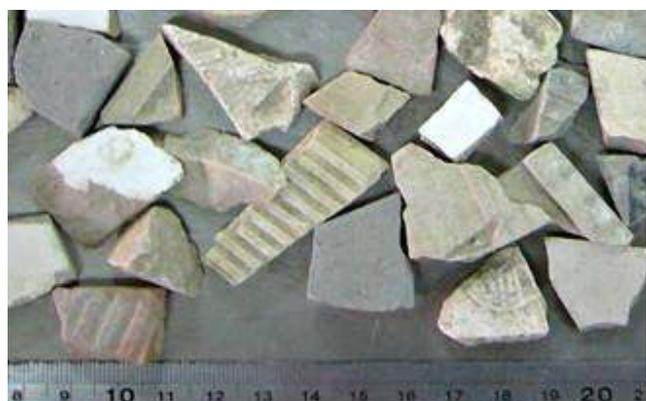
Figure 2 Recycled tile aggregate
