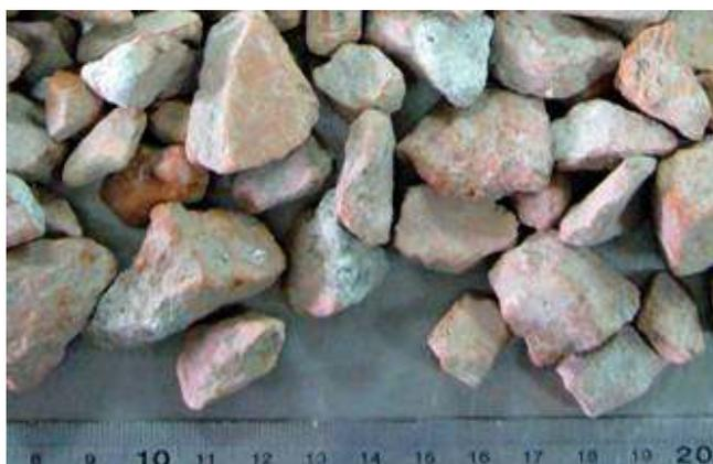
Figure 1 Recycled brick aggregate
