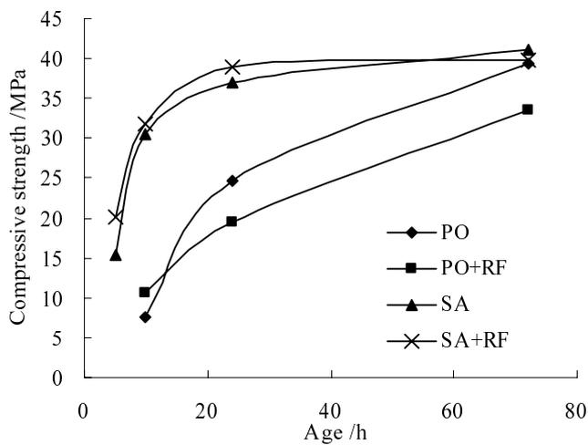
Figure 6. Early compressive strength of concrete.
