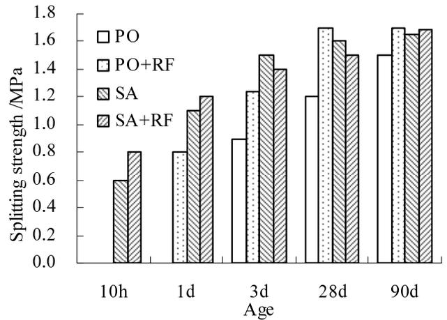
Figure 7. Interfacial bond strength of concrete.
