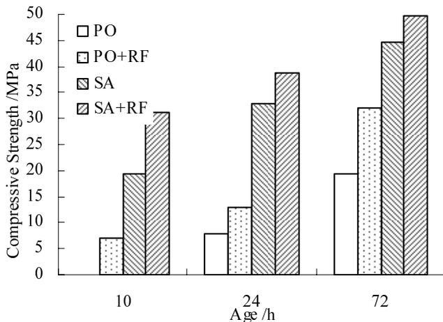
Figure 2. Early compressive strength of cement mortar using RF.
