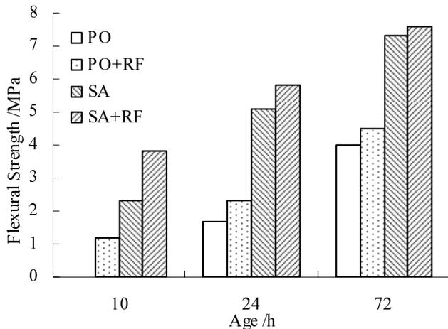
Figure 1. Early flexural strength of cement mortar using RF.
