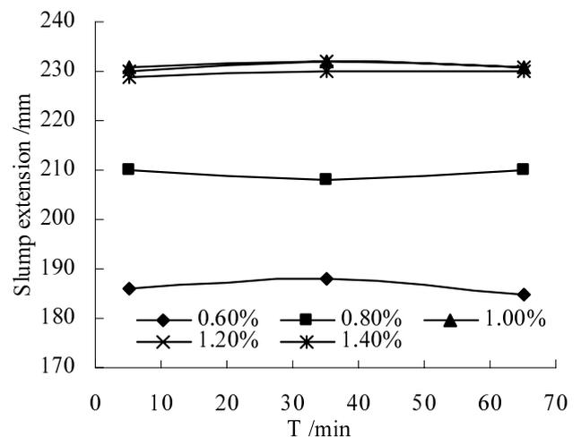
Figure 4. Slump extension of cement mortar without RF admixture.
