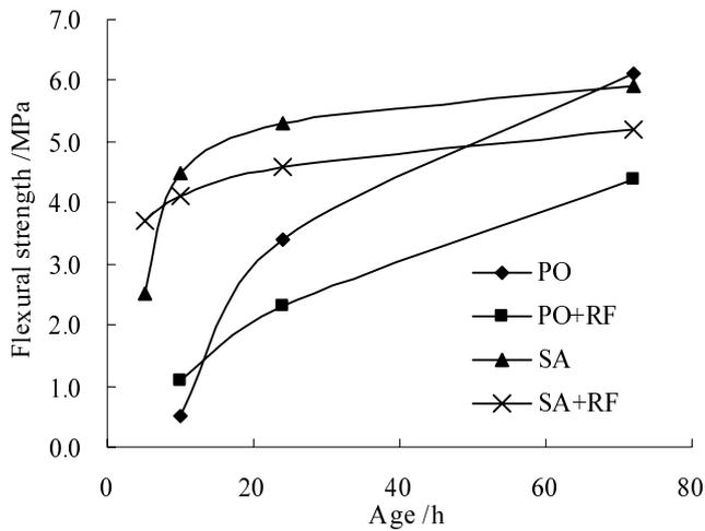
Figure 5. Early flexural strength of concrete.
