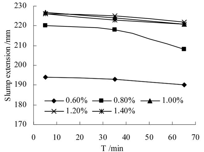
Figure 3. Slump extension of cement mortar using RF admixture.
