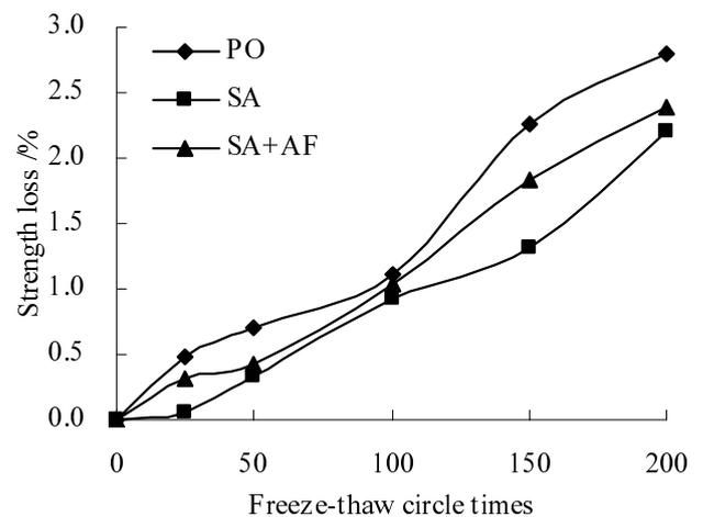
Figure 8. Freeze-thaw durability of concrete.
