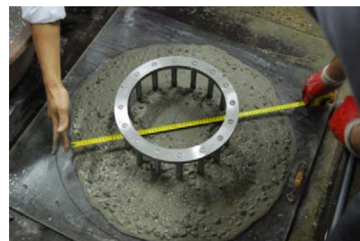
Figure 3. J-Ring test of fresh concrete.
