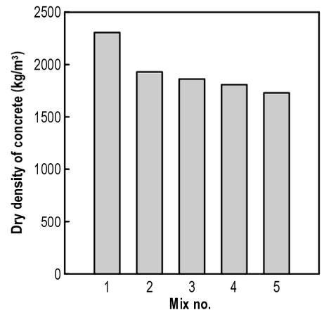
Figure 7. Dry density of SCC.
