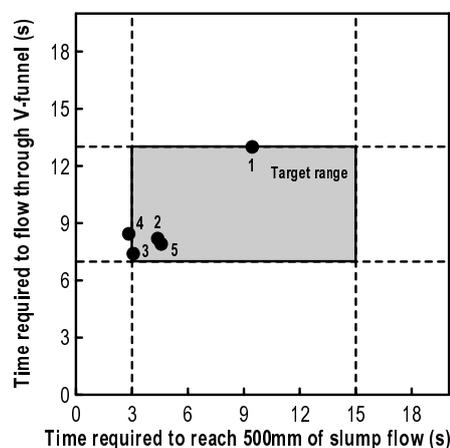
Figure 2. SCC segregation resistance ability.
