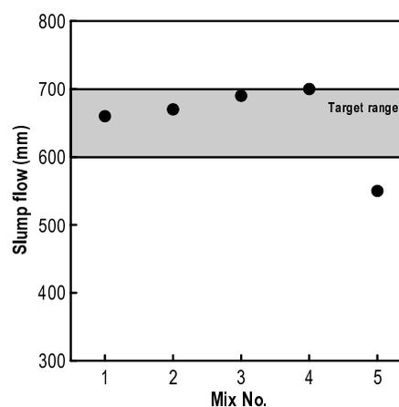
Figure 1. Slump flow results.
