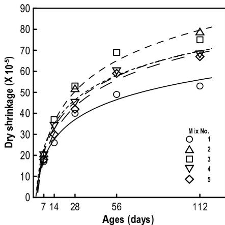
Figure 8. Dry shrinkage of SCC.
