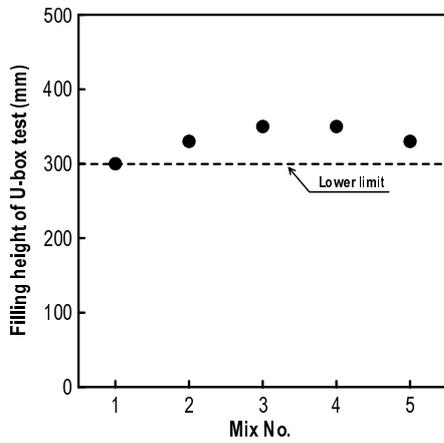
Figure 3. Filling height of U-box test.
