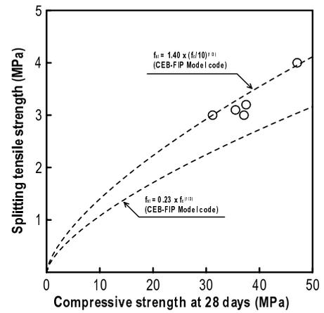
Figure 5. Relationship between compressive strength and splitting tensile strength.
