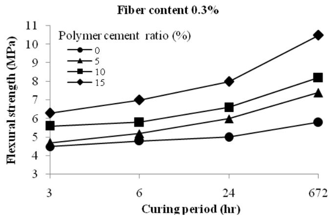
Figure 3. Curing period Versus Flexural Strength of Ultrarapid-Hardening Polymer-Modified Concretes with fiber content
