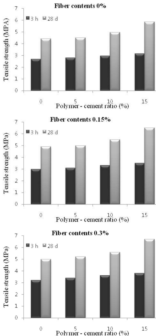
Figure 5. Curing Period Versus Tensile Strength of Ultrarapid-Hardening Polymer-Modified Concretes with fiber content
