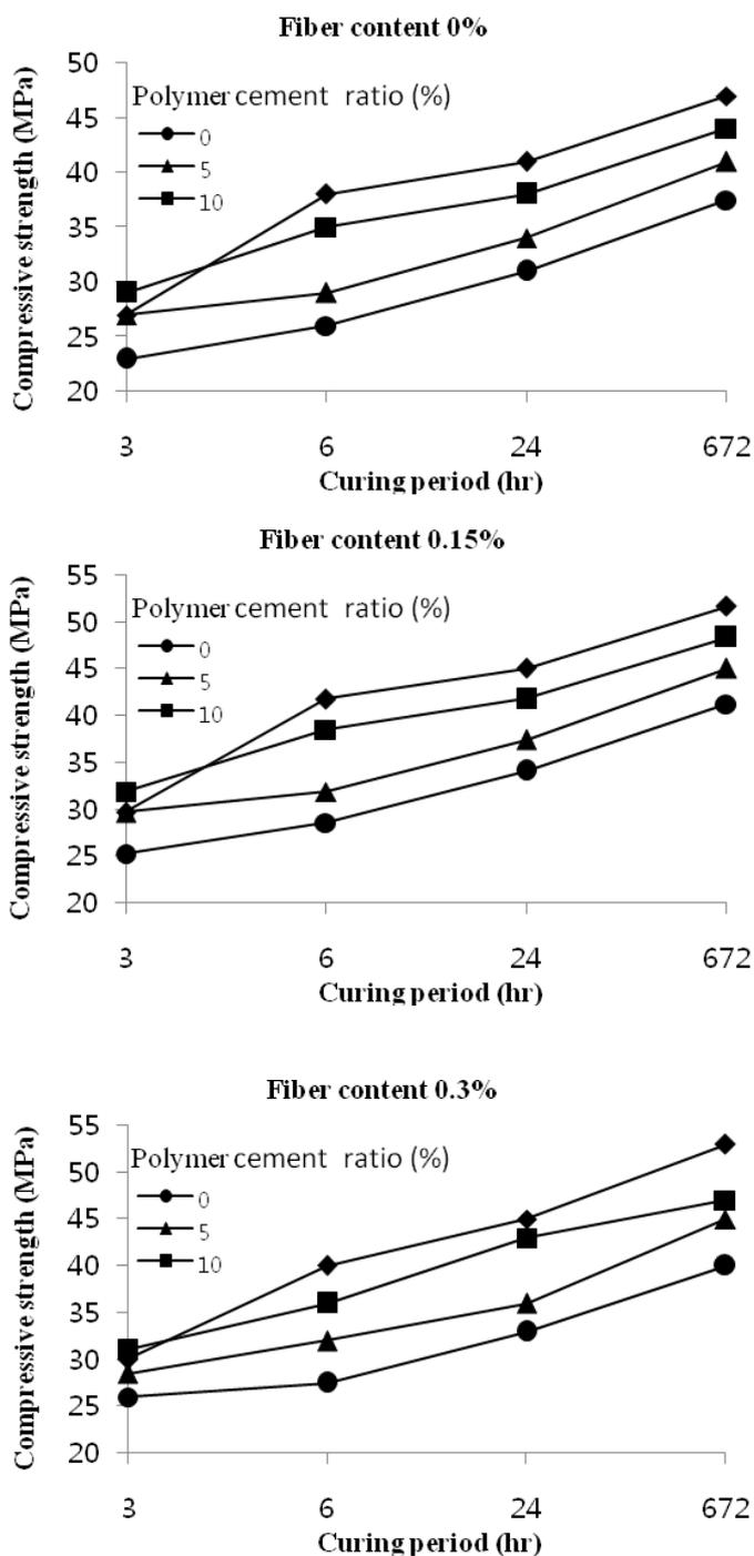
Figure 4. Curing Period Versus Compressive Strength of Ultrarapid-Hardening Polymer-Modified Concretes with fiber content
