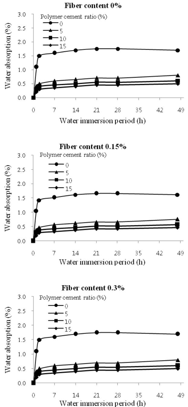
Figure 2. Immersion period Versus water absorption of Ultrarapid-Hardening Polymer-Modified Concretes with fiber content
