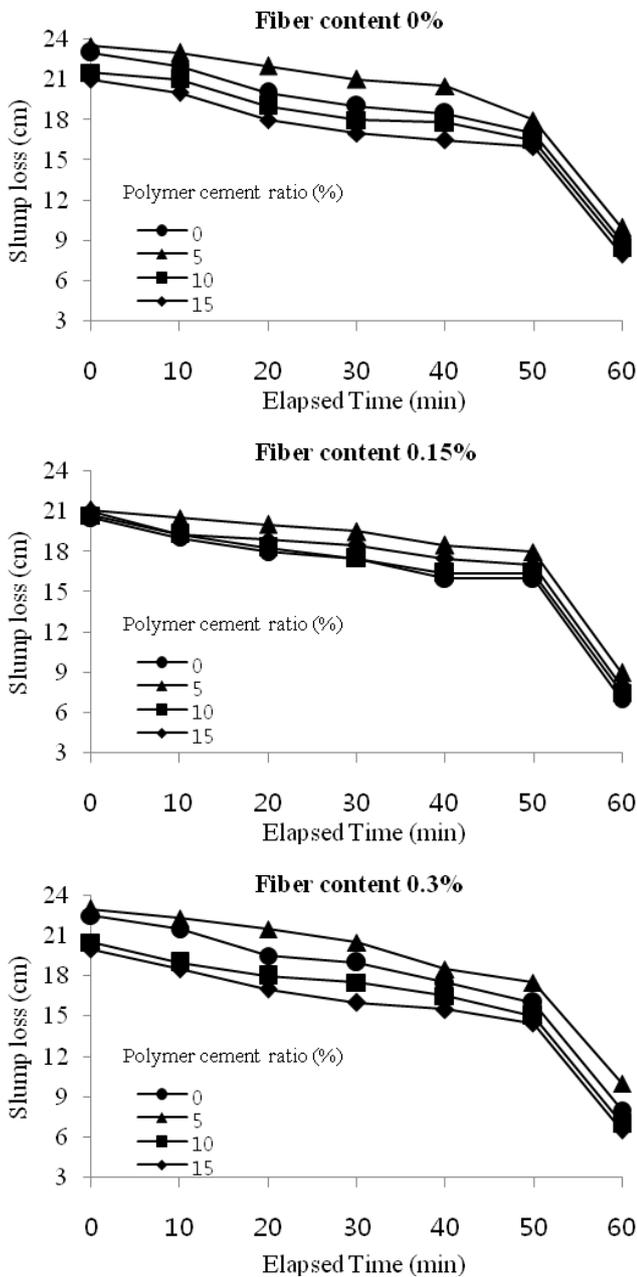
Figure 1. Elapsed Time Versus Slump Loss of Ultrarapid-Hardening Polymer-Modified Concretes with fiber content
