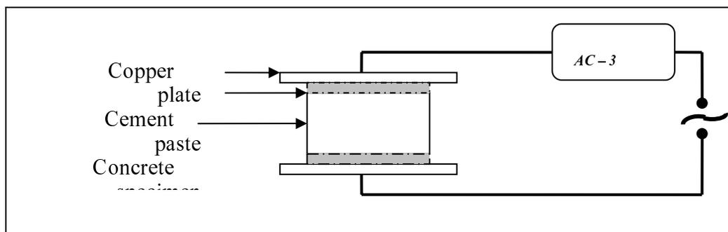
Figure 3. Electrical resistivity measuring instrument.
