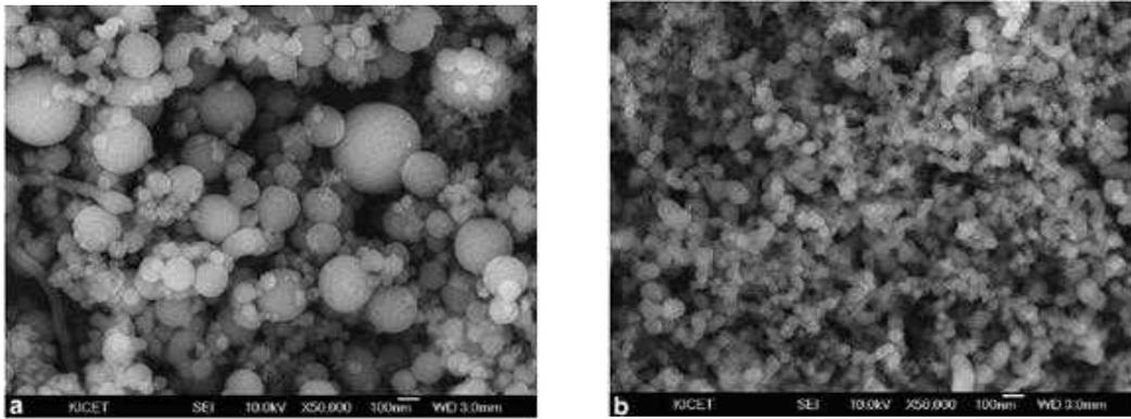
Figure 1. SEM photographs of materials: (a) silica fume (b) nano-SiO<sub>2</sub> [9].
