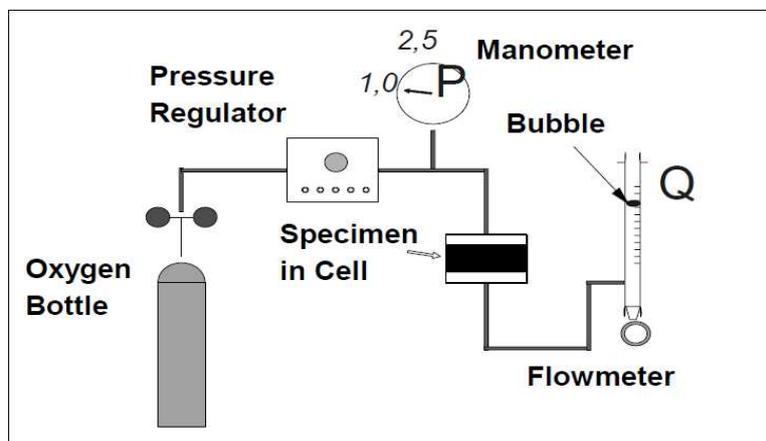
Figure 2. Details of gas permeability device [14].
