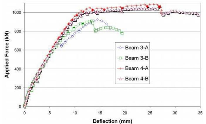
Figure 6. Load-deflection curves of reinforced beams.
