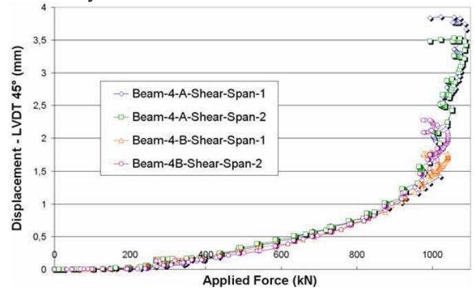
Figure 11. Displacement measured by LVDT sensors fixed at 45° - Load curves of reinforced beams with stirrups.
