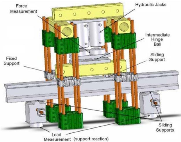
Figure 3. Overview of the specimen under four point bending test.
