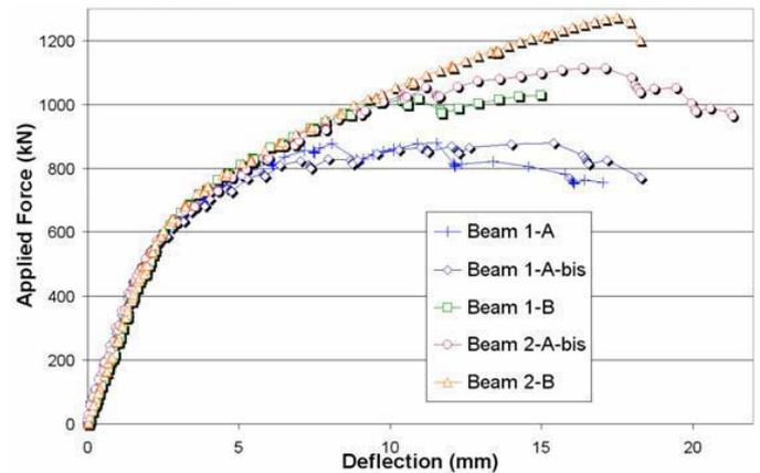
Figure 5. Load-deflection curves of prestressed beams.
