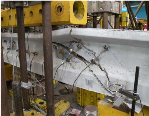
Figure 7. Shear failure of Beam 1-B.
