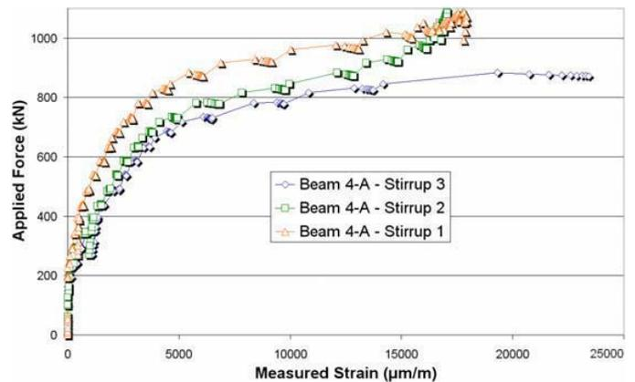
Figure 12. Strain development in stirrups for beam 4-A.
