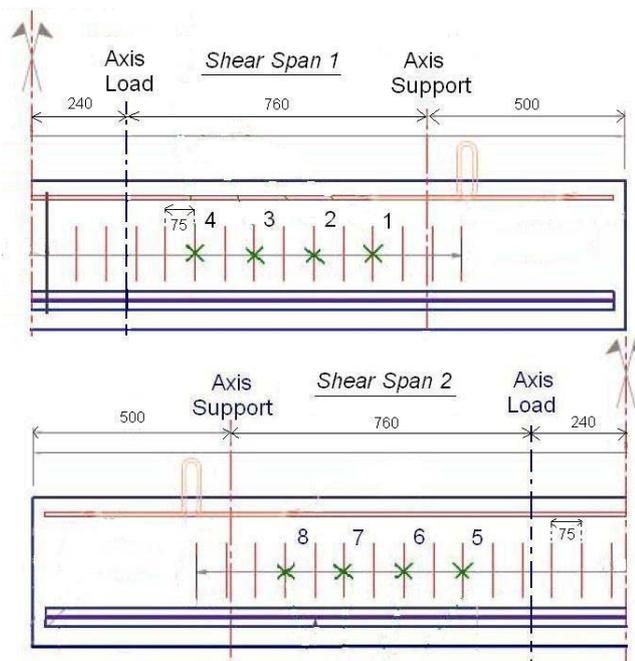
Figure 4. Locations and reference number of stirrups on which strain gauges were attached. (Dimensions in mm).
