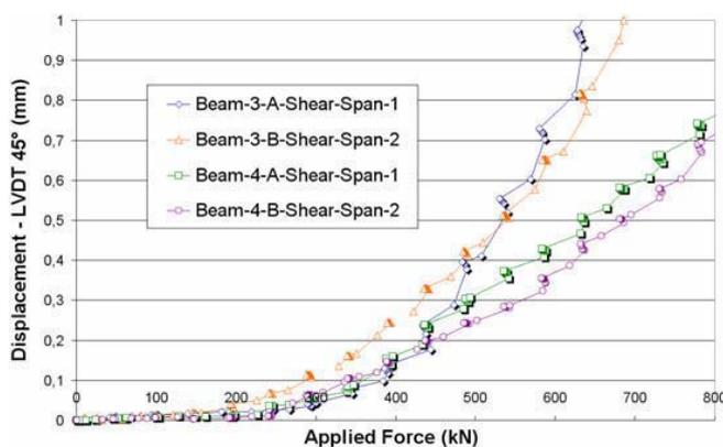
Figure 15. Displacement measured by LVDT sensors fixed at 45°- Load curves of reinforced beams with and without stirrups.
