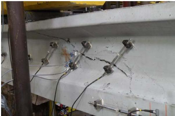
Figure 9. Shear failure of Beam 3-A.
