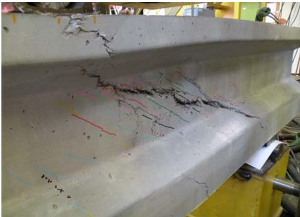
Figure 8. Shear failure of Beam 2-A-bis.
