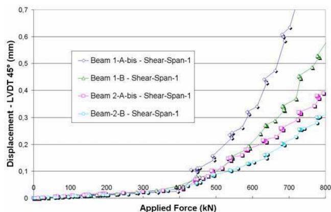
Figure 14. Displacement measured by LVDT sensors at 45°- Load curves of prestressed beams with and without stirrups.
