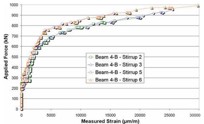
Figure 13. Strain development in stirrups for beam 4-B.
