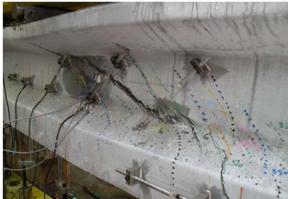
Figure 10. Shear failure of Beam 3-B.
