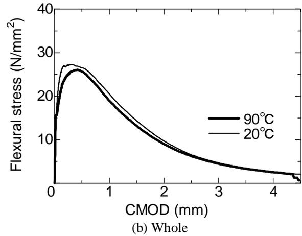
Figure 4. Load-CMOD curves with different curing temperature.
