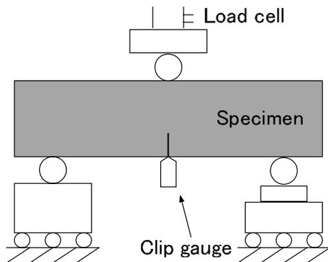
Figure 3. Bending test.
