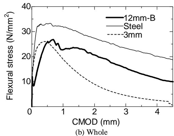
Figure 6. Load-CMOD curves with different kind of fiber.
