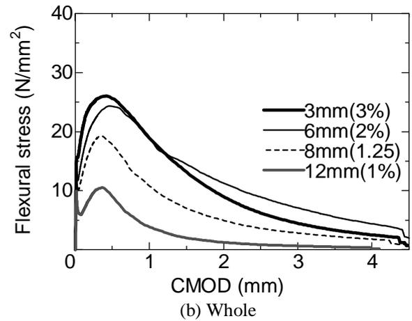
Figure 5. Load-CMOD curves with different length of fibers.
