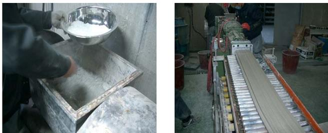
(a) Dry mixing (b) Extruding process of ECC panel
