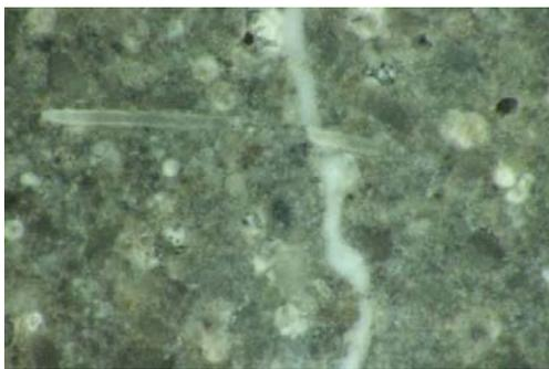
Figure 15. Crack opening closure after permeability test.
