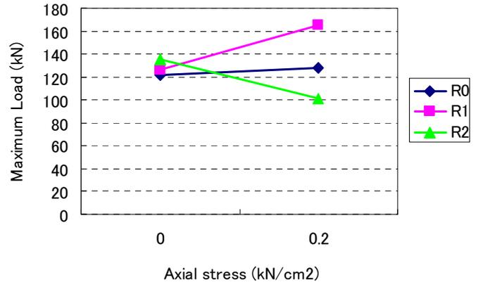
Figure 8. Relationship between ultimate strength and axial compression.
