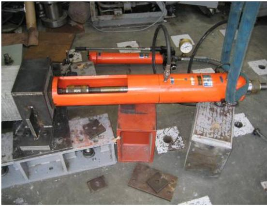
Figure 6. A jack for axial tensile compression.
