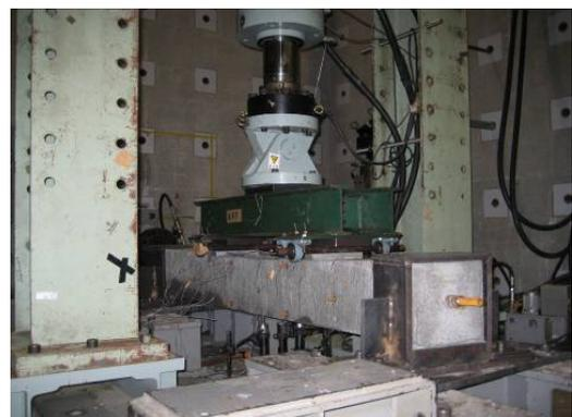
Figure 4. Test apparatus and bending test of a curved beam.
