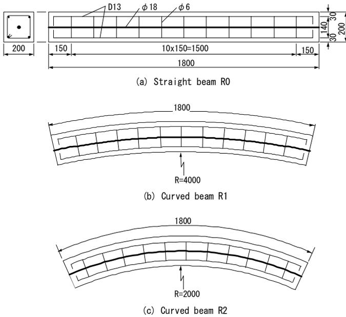
Figure 2. Cross-section of a curved beam.
