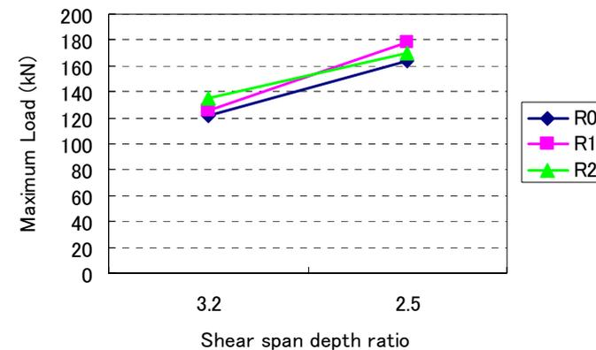
Figure 7. Relationship between ultimate strength and a/d.
