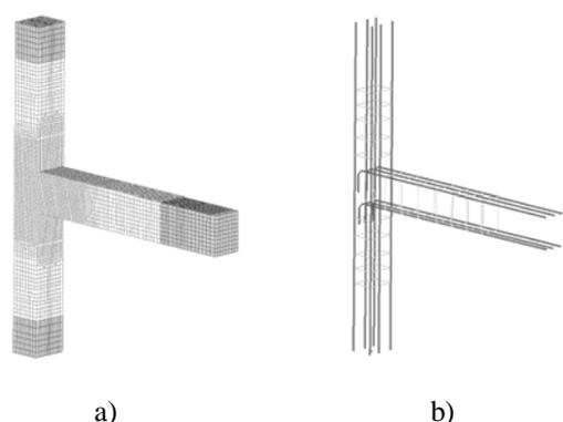
Figure 7. FE Model (JT4-1): a) Discretization of concrete; b) Discretization of reinforcement.
