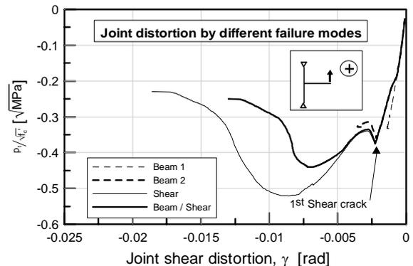
Figure 17. Interaction between beam flexural failure and joint shear cracking. ( $p_j - \gamma$  curves)
