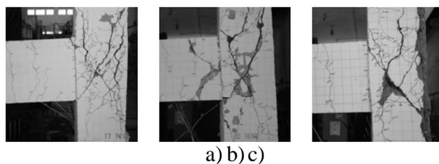
Figure 5. Cracking pattern at end of the tests: a) JT1-1; b) JT3-1; c) JT4-1.
