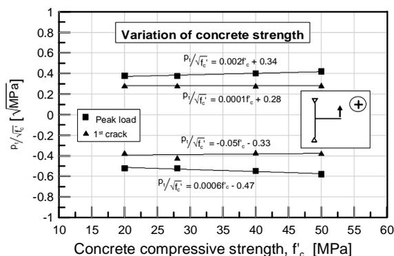
Figure 12. Effect of variation of concrete strength on the joint shear capacity.
