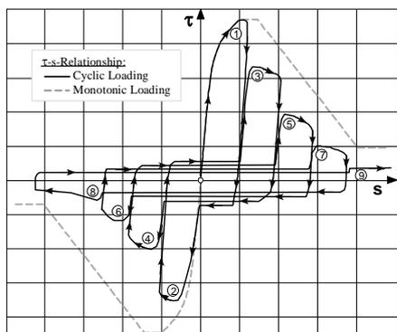
Figure 6. Bond-slip cyclic relationship for deformed bars (Eligehausen et al. 1983).
