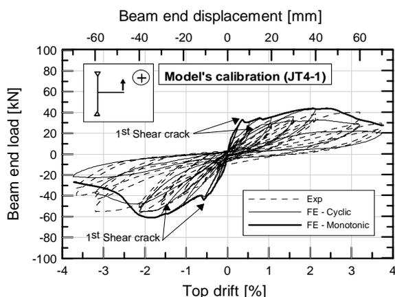
Figure 8. Comparison between numerical and experimental results: Hysteretic behavior of specimen JT4-1.
