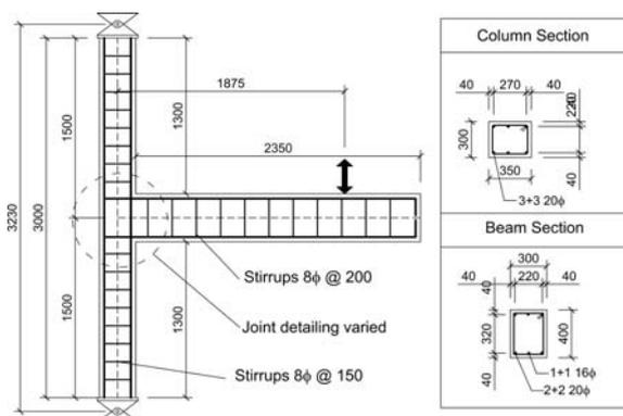
Figure 2. Geometry and reinforcement of the test specimens.
