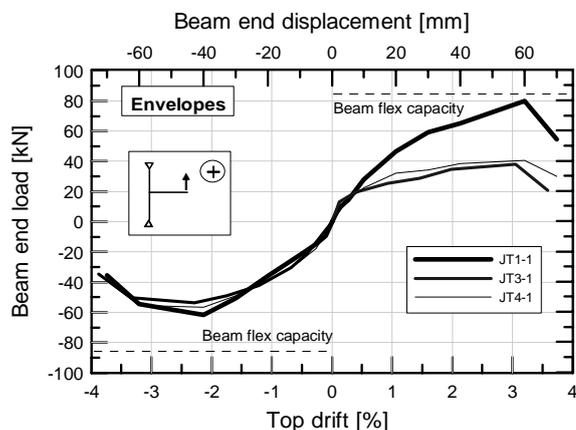
Figure 4. Envelopes of hysteretic cycles observed in the experimental tests.
