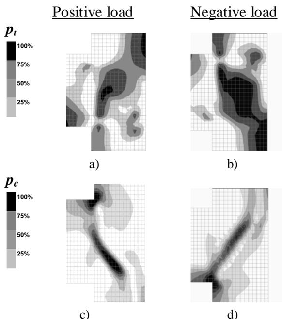
Figure 11. a), b) Tensile stresses in the core at 1<sup>st</sup> shear crack; c), d) Compressive stresses in the core at peak load.
