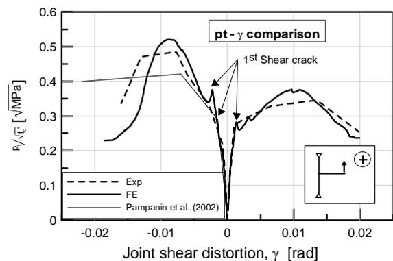
Figure 9. Comparison between numerical and experimental results: Joint deformation.
