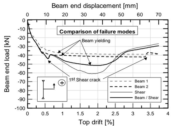
Figure 16. Interaction between beam flexural failure and joint shear cracking (load displacement curves).
