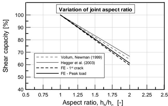
Figure 15. Variation of aspect ratio ( $h_b / h_c$ ) for the case of bars bent into the joint.
