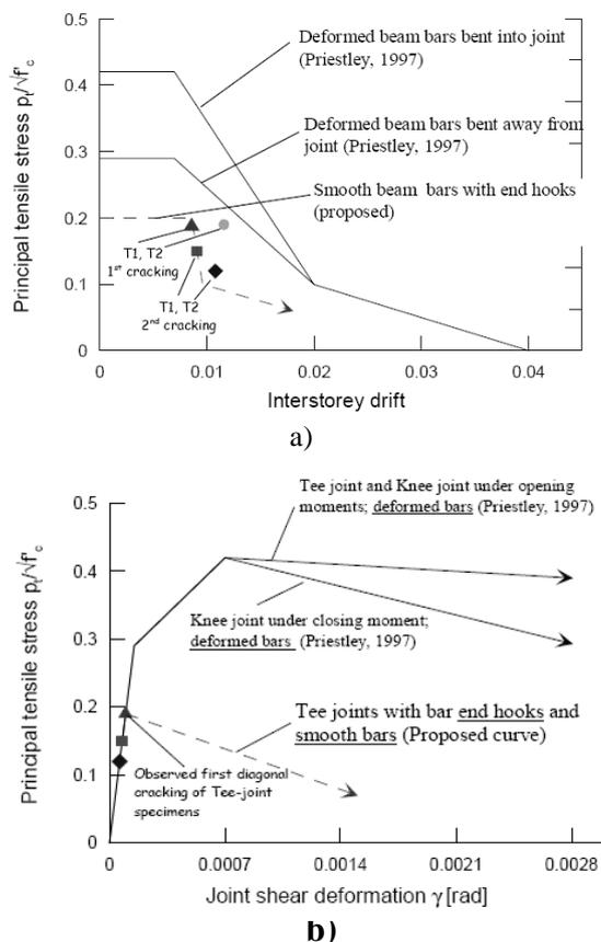
Figure 1. a) Joint shear capacity as function of the top drift; b) Joint shear capacity as function of the joint shear deformation (Priestley (1997), Pampanin et al. (2002)).
