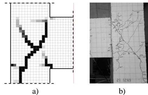
Figure 10. Comparison of cracking of the joint panel in specimen JT4-1 at approx. 30 mm displacement: a) Numerical simulation; b) Experimental test.
