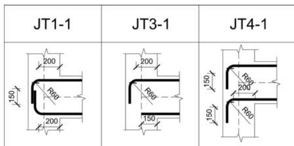
Figure 3. Beam bars anchorage for the different specimens.
