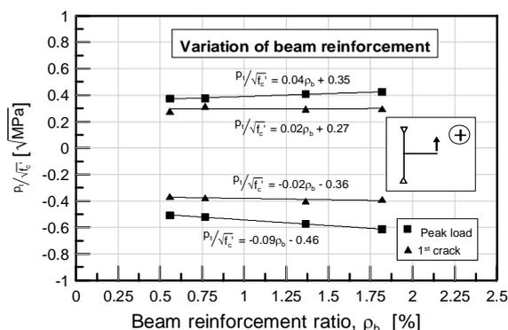
Figure 13. Effect of variation of beam reinforcement on the joint shear capacity.
