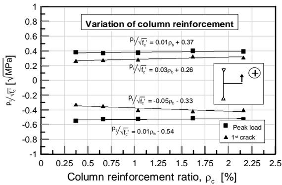
Figure 14. Effects of variation of column reinforcement on the joint shear capacity.
