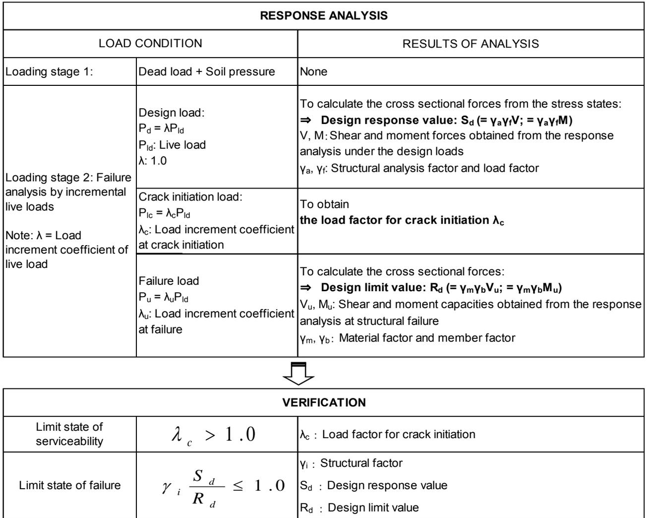
**Figure 6:** Design flow chart based on the response analysis
