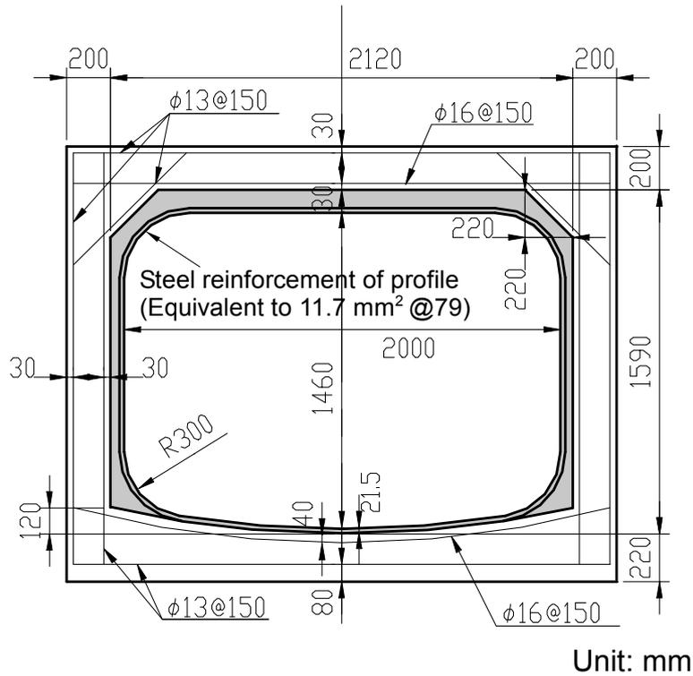
Figure 7: Dimensions of an aging sewer after renovation
