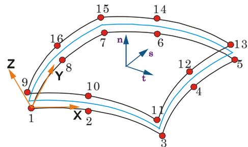
**Figure 5:** Schematics for 16 node interface element
