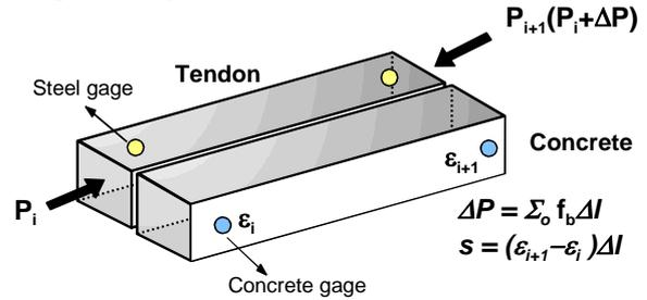
Figure 1: Measurement of bond stress and slip
