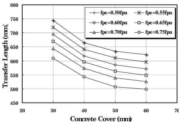
**Figure 9:** Comparison of transfer length according to concrete cover
