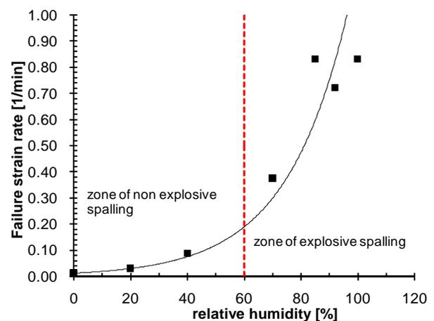
Figure 7: Variation of failure strain rate with RH.
