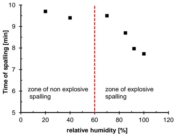
Figure 8: Variation of time of spalling with RH.
