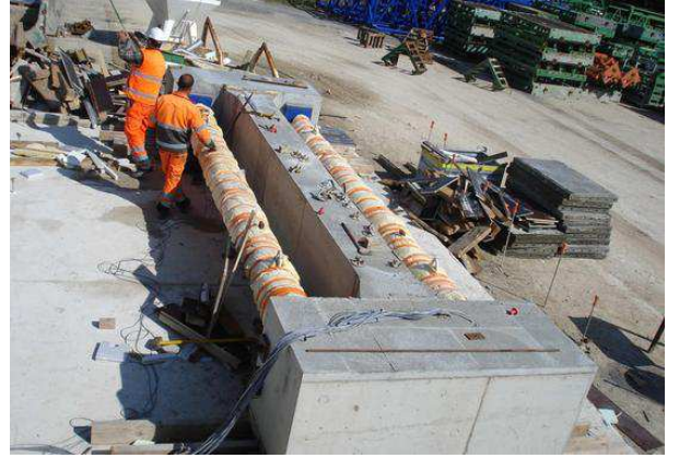
Figure 1: A validated massive beam RG8 with restrained shrinkage (image and data from the database Cheops).
