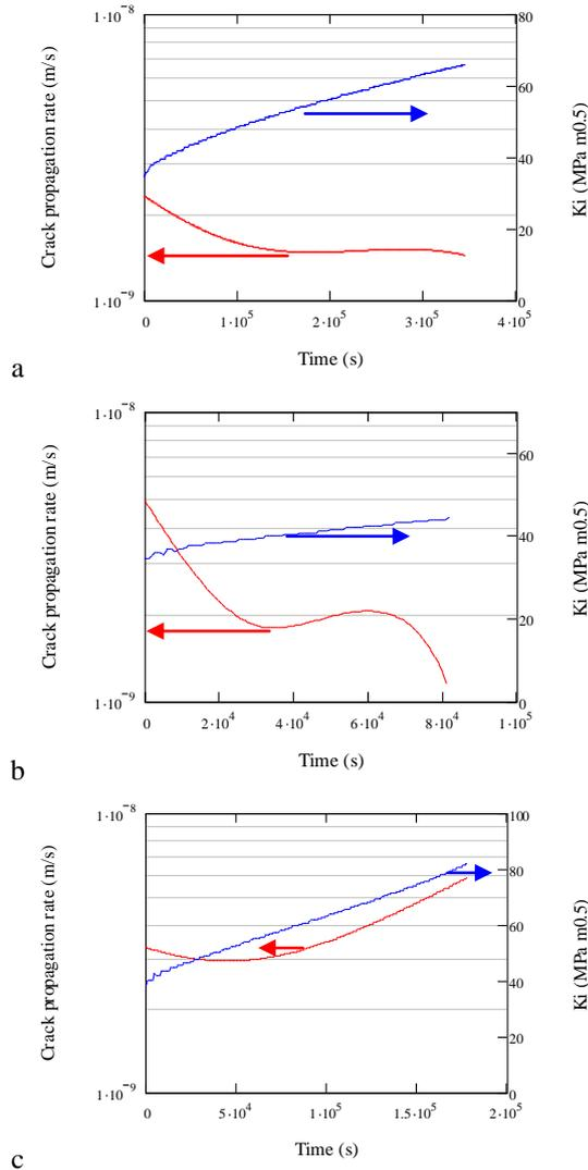
**Figure 4:** Crack Propagation Rate calculated from the model and test reference in table 2: a) crack growth rate of T04 test, b) crack arrest of test A05, and c) fracture of A07 specimen during the test.
