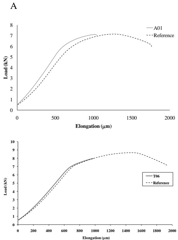
**Figure 2:** Mechanical behavior of steel after crack generation test.
