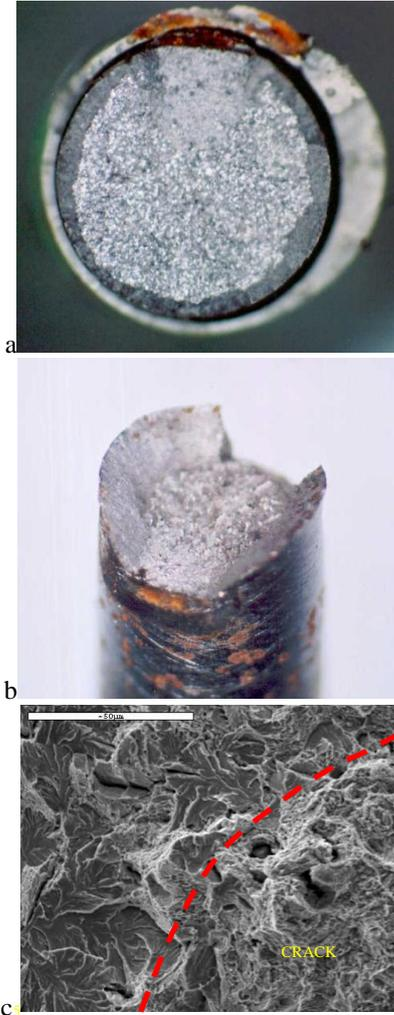
**Figure 3:** Surface of fracture: a) modified parent pearlitic steel, b) cold drawn steel and c) Crack tip.
