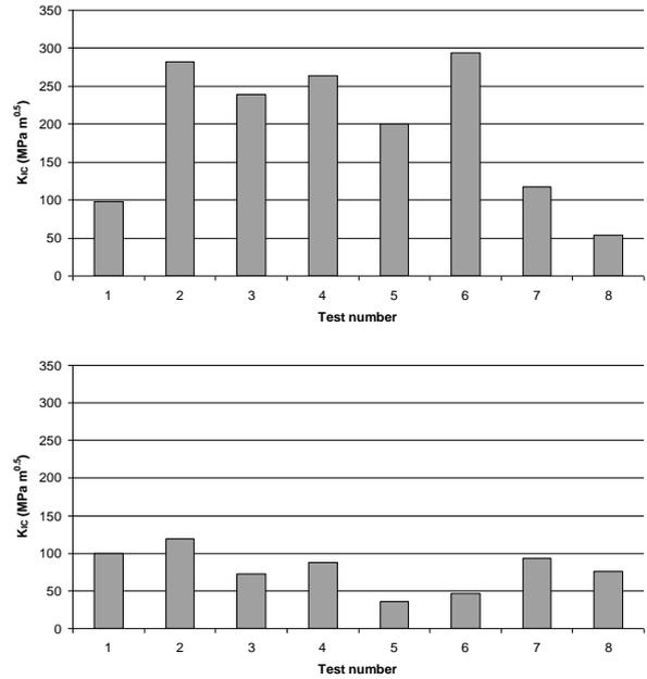
**Figure 5:** Fracture toughness of cold drawn steel (top) and parent steel (down) after stress corrosion cracking test.
