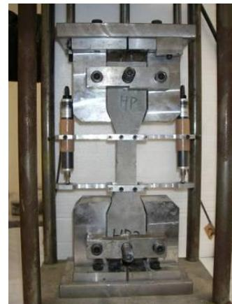
**Photo 1:** Uniaxial tension testing apparatus
