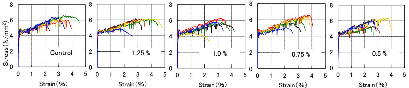
**Figure 4:** Stress-strain relationship of Series 3 by uniaxial tension testing
