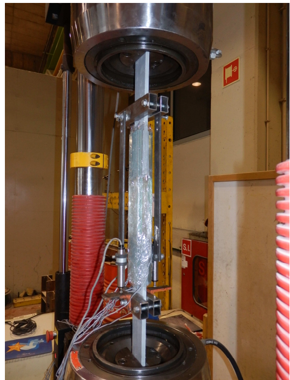
Figure 1: Double lap joint specimen during tensile test.
