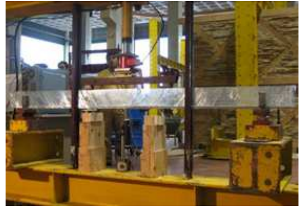
Figure 4: Configuration scheme of the bending tests on a glass beam strengthened with GFRP [3].
