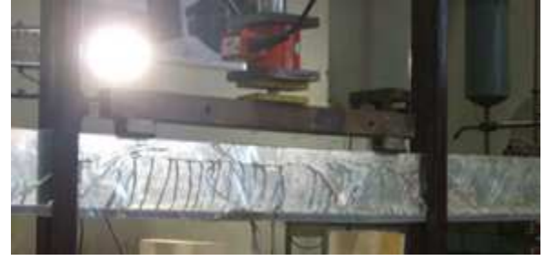
Figure 11: Beam crack pattern [3].
