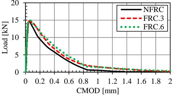
**Figure 7:** Load-CMOD curves of FRCs versus control
