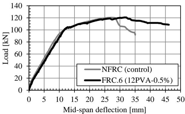
**Figure 8:** Load-deflection curves of PVA-FRC beam versus control
